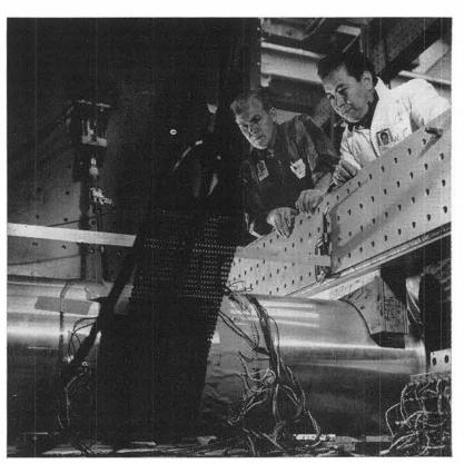
ALUMINUM CYLINDER will be tested to determine breaking point. Force is exerted by hydraulic cylinders to the wire mesh strap under the cylinder. Data will be measured by transducers attached to the test specimen. Checking setup are Harry Warrick and Gil Leyba.
